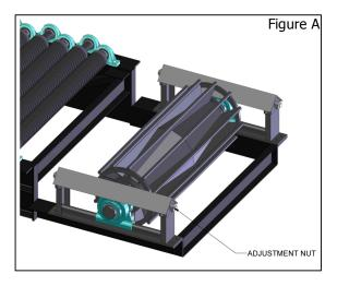
and get help if necessary to remove any guards. Use a wrench and insure that you only apply enough belt tension such that the belt does not slip around the drive pulley. In most conveyor installations, mechanical take-up units are also used to adjust belt tracking.
